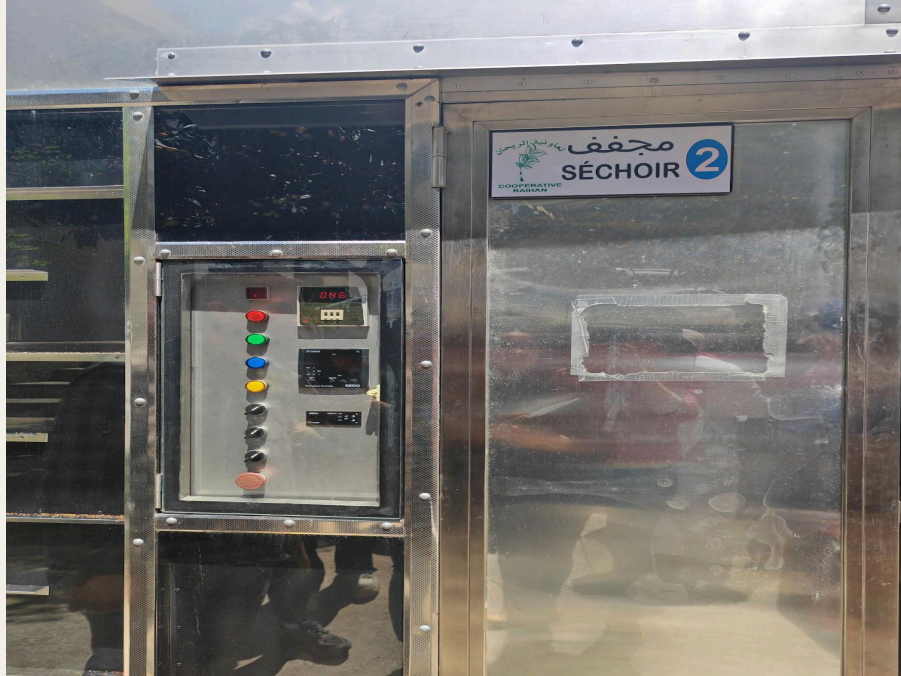
Controller of the Solar Drying Chamber. Photo: Xiao Chenjuan.
